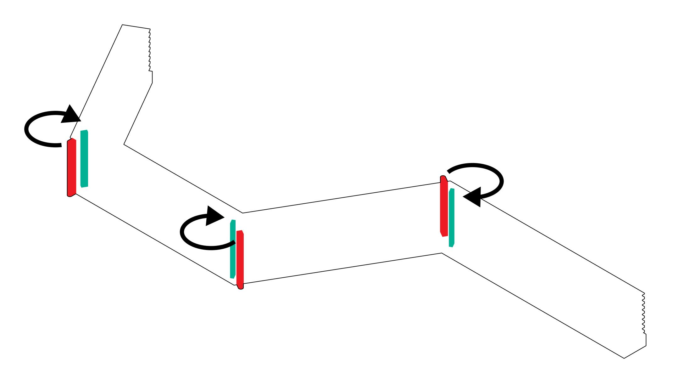
concrete additions removed: new elevators placed inside the existing cores
